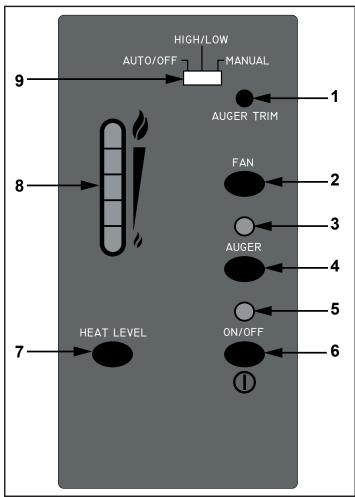
Figure 3: Circuit Board Control Panel Decal
